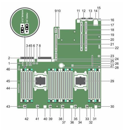
Figure 60. System board connectors and jumpers
